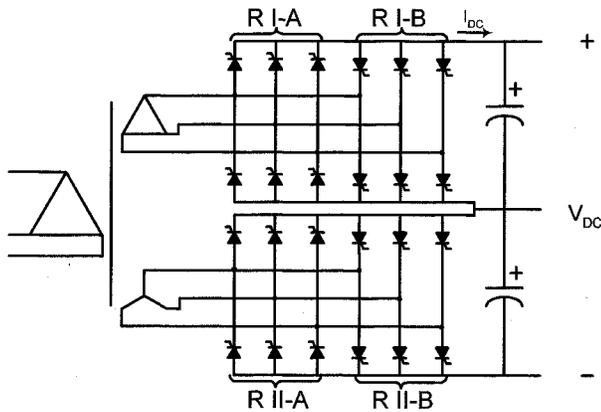
Fig. 8. Line-side dual converter for a three-level inverter.
