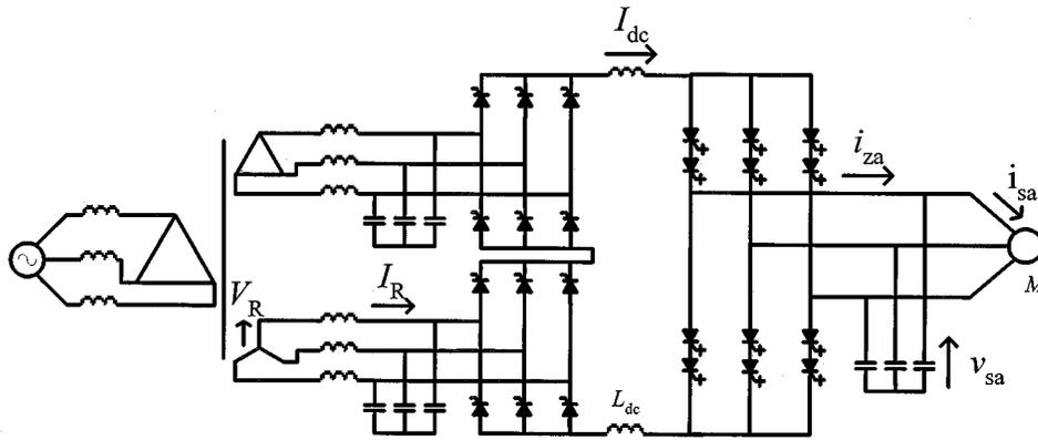
Fig. 5. Power circuit of the PWM-CSI inverter.
