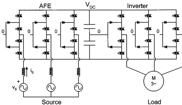
Fig. 9. Power circuit of GTOs three-level AFE-inverter.
