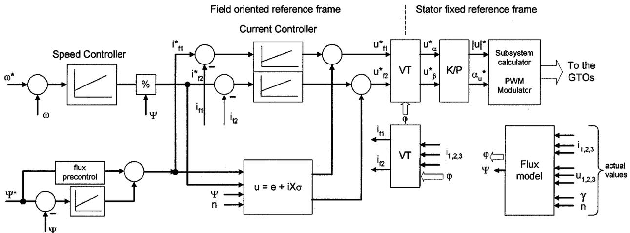
Fig. 6. Control of the inverter and the machine.
