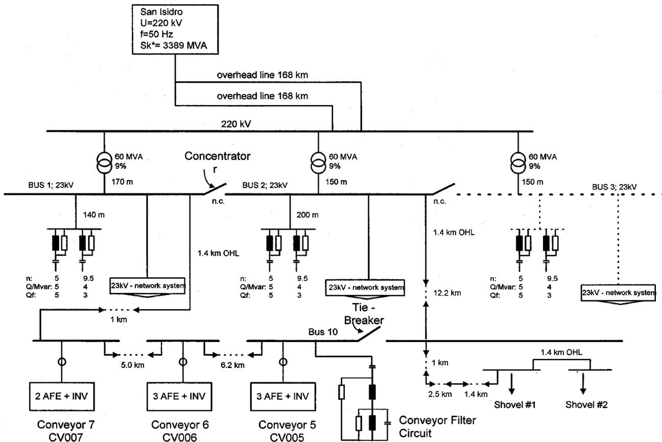
Fig. 7. Simplified single-line diagram for harmonics study.
