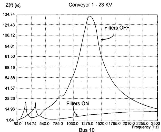
Fig. 8. Behavior of the impedance  $Z(f)$  of bus 10, 23 kV with tie breaker open.
