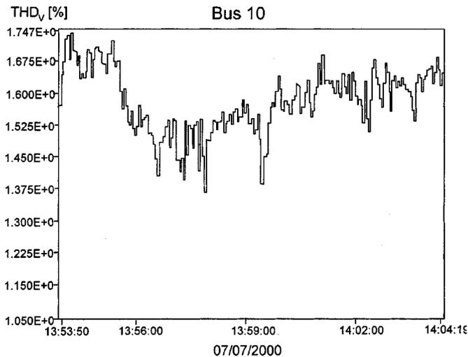
Fig. 11. Measured distortion ( $THD_v$ ) of bus 10 with conveyor filter.
