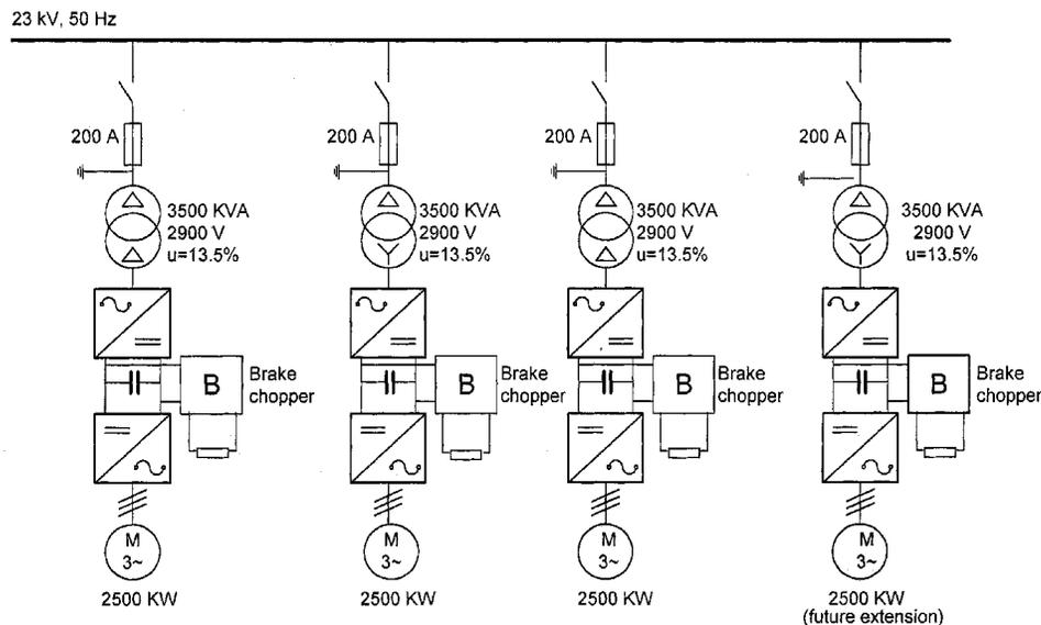
Fig. 3. Drive station with four motors (final extension).
