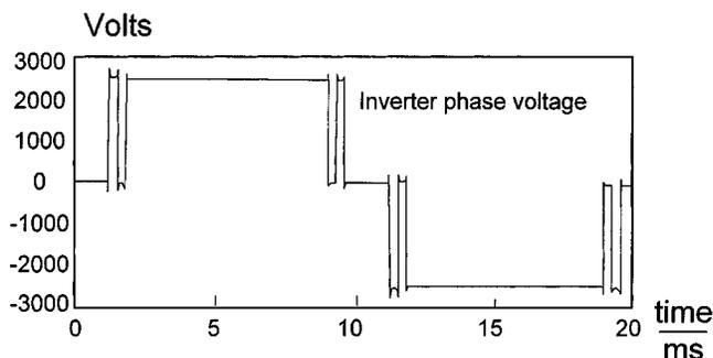
Fig. 4. Phase voltage of a single AFE.
