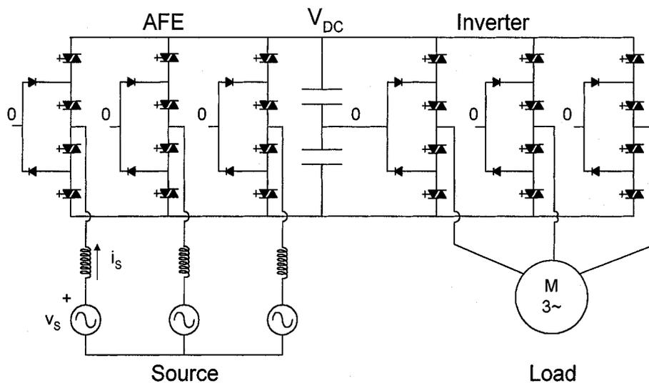
Fig. 2. Power circuit of the three-level inverter-AFE system.
