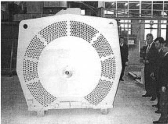
Fig. 1. 2500-kW conveyor motor.
