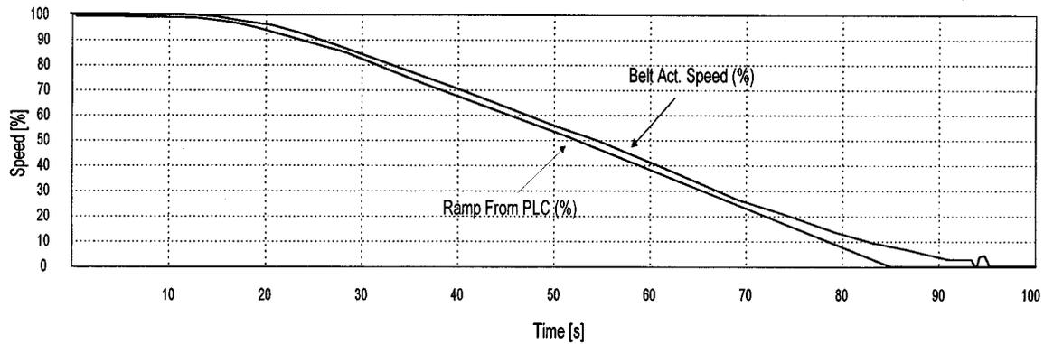
Fig. 9. Measured braking curve of the belt.
