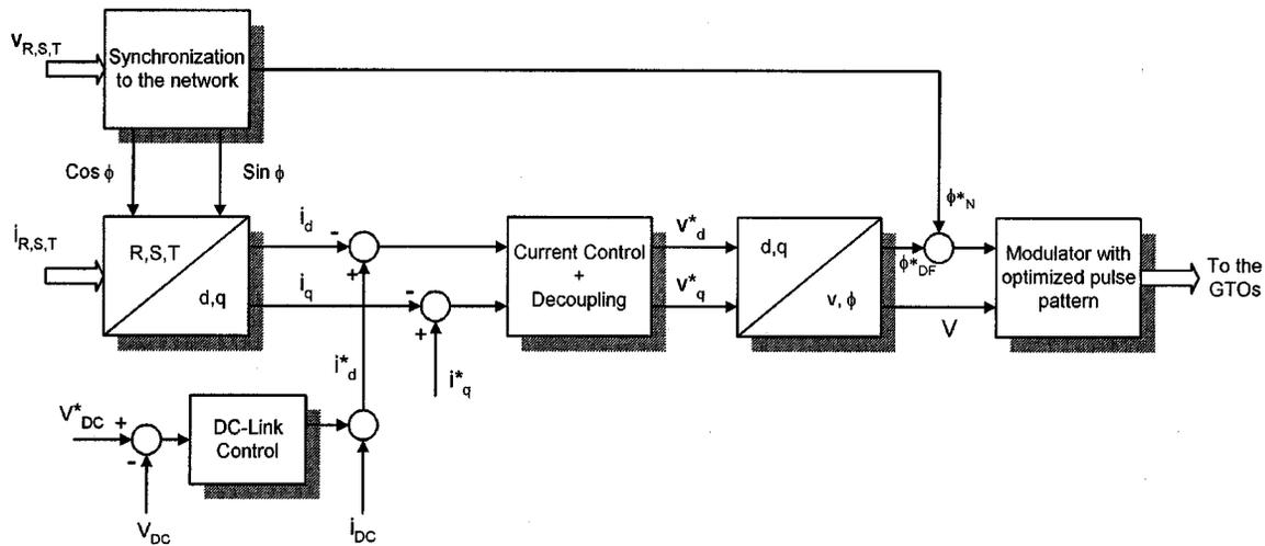
Fig. 5. Simplified structure of the AFE control.
