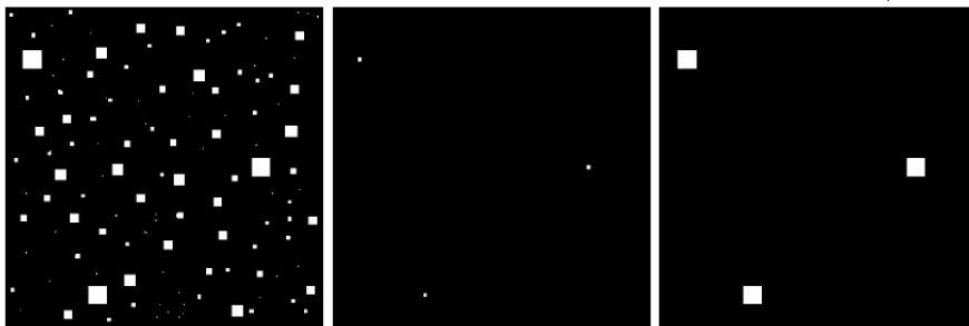
FIGURE 9.7 (a) Image of squares of size 1, 3, 5, 7, 9, and 15 pixels on the side. (b) Erosion of (a) with a square structuring element of 1's, 13 pixels on the side. (c) Dilatation of (b) with the same structuring element.
