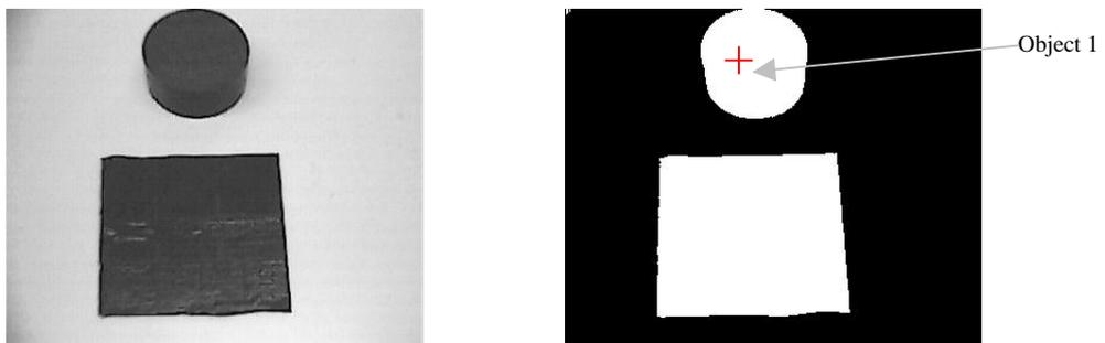
**Figure 20.** a) Grayscale image and b) binary image.
