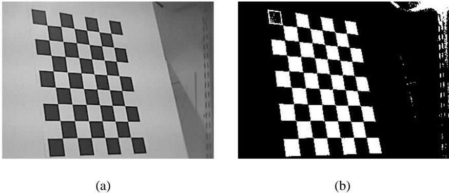
**Figure 18.** a) Grayscale image and b) binary image.
