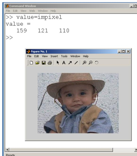
**Figure 6.** Use of the function `impixel`.
