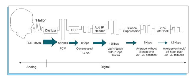
Figure 18 - VoIP Bandwidth Reduction Sequence
