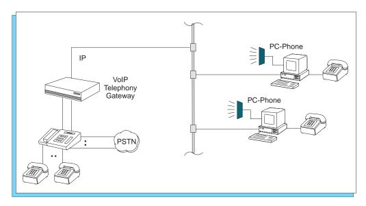
Figure 22 - PC Phone using VoIP Gateway
