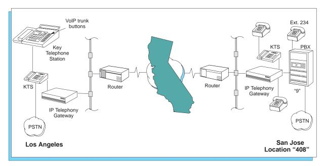
Figure 12 - Calling from a KTS using VoIP
