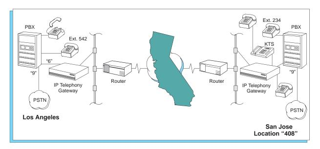
Figure 11 - Calling from a PBX using VolP
