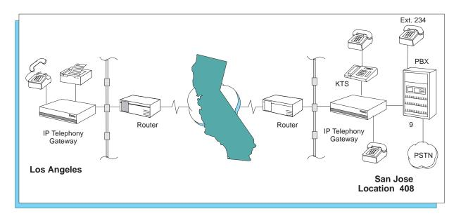
Figure 13 - Calling from a directly connected phone using VoIP
