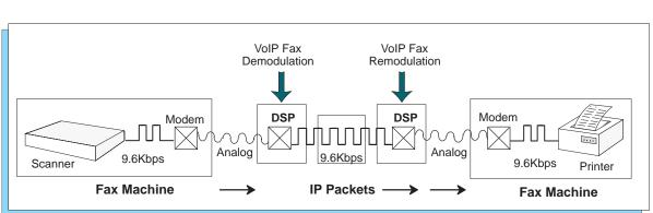
remodulated back into the original analog fax signal by the remote gateway, for delivery to the remote fax machine.
