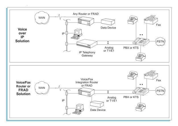
Figure 10 - Comparing VoIP Gateway with Voice/Fax Router or FRAD
