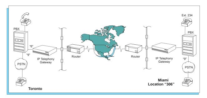
Figure 14 - Off-net calling using VoIP
