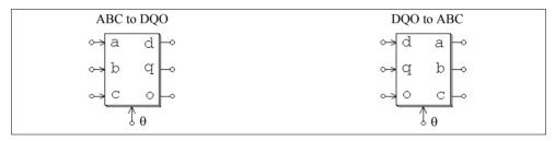
It should be noted that, in the power circuit, currents must first be converted into voltage quantities (using current-controlled voltage sources) before they can be transformed. Also, if an input terminal is not used (such as in the DQO-to-ABC transformation block where only Phase D and Q are not used, and Phase O is not used), it must be connected to ground.
