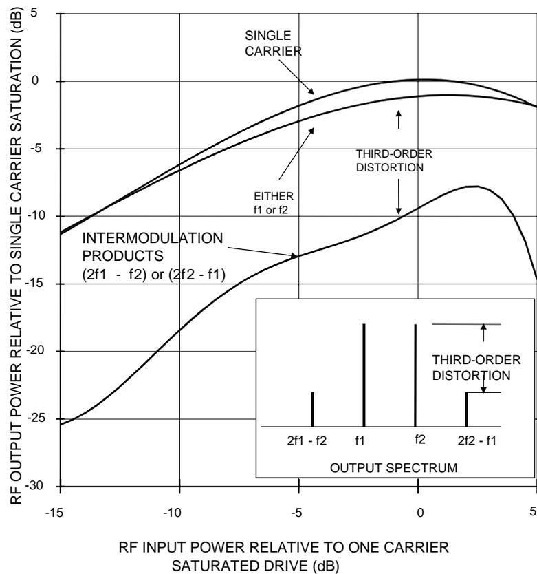
**Figure 5.7 Typical Third-Order Intermodulation Data for TWTA**
