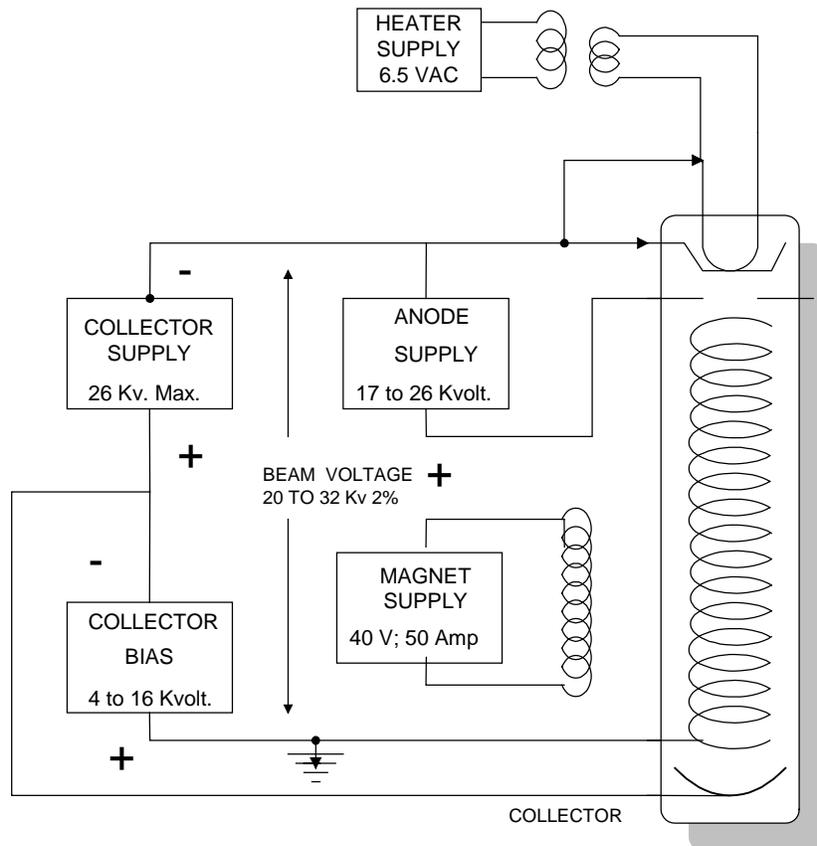
**Figure 5.6 Depressed Collector Power Supply**
