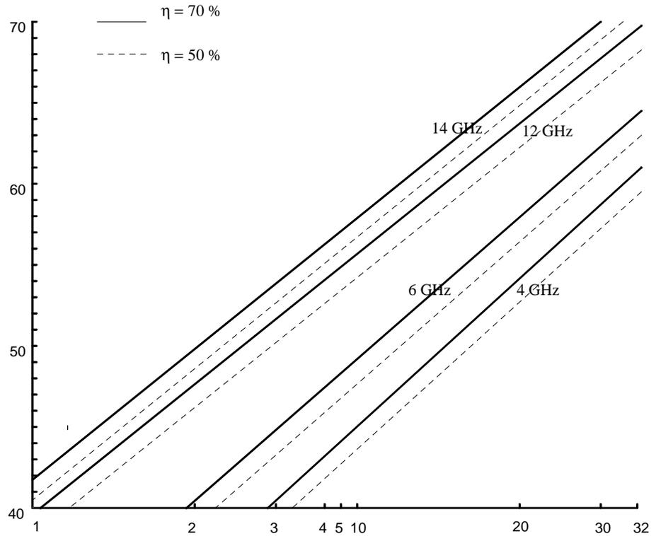
Figure 3.10 Antenna Gain vs. Diameter
