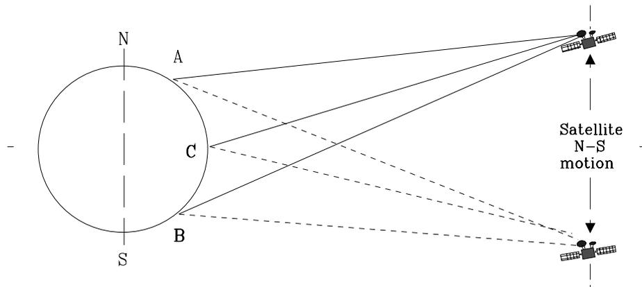
**Figure 4.2 Impact of Orbital Inclination over Link Length**
