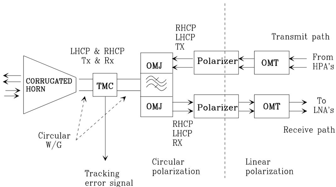
**Figure A.8 Typical Four-Port Feed System Block Diagram**
