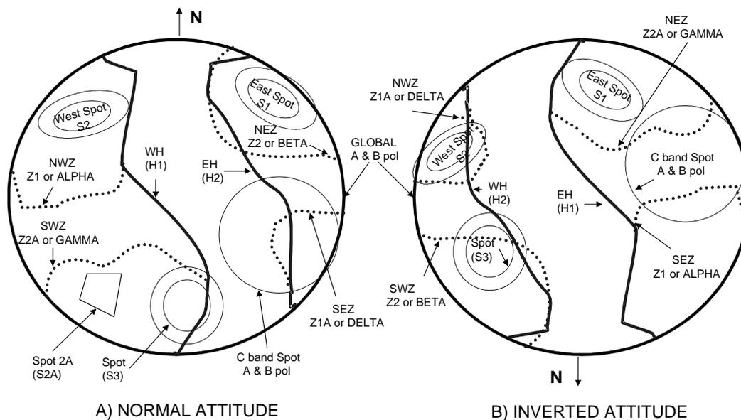
Figure 2.10 INTELSAT VII Typical Beam Coverage
