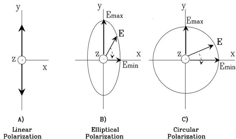
**Figure A.13 Linear, Elliptical, and Circular Polarization**
