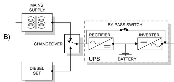
**Figure 10.7 Power Plant Standby Diesel with No-Break**
