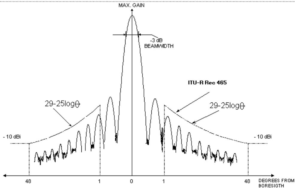
**Figure 3.9 Antenna Radiation Diagram and Beamwidth**
