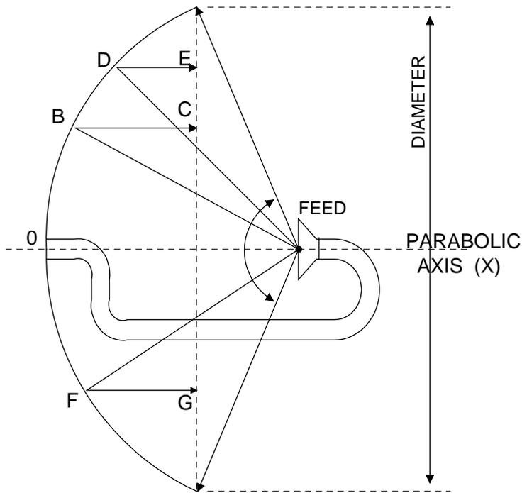
**Figure 3.1 Center Feed Antenna**
