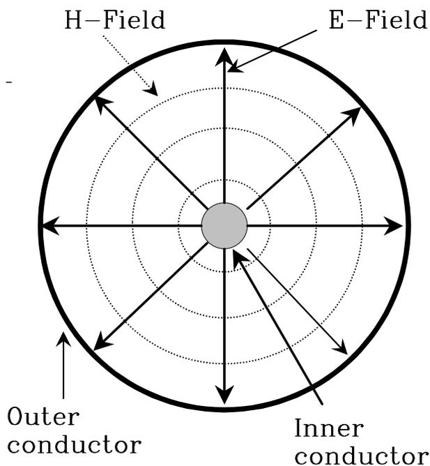
**Figure A.3 TEM Wave in a Coaxial Cable**
