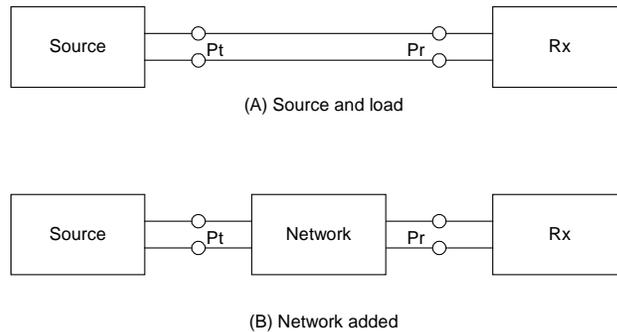
**Figure 8.6 Insertion Loss or Gain**
