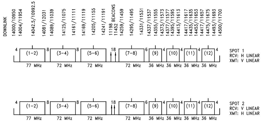
Figure 2.17 INTELSAT IX Transponder Layout (Ku-band)
