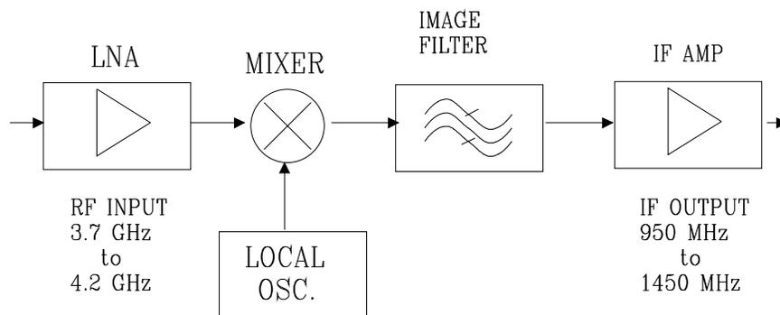
**Figure 6.3 Block Diagram of an LNB**
