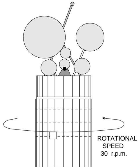
**Figure 2.4 Cylindrical Spin-Stabilized**
