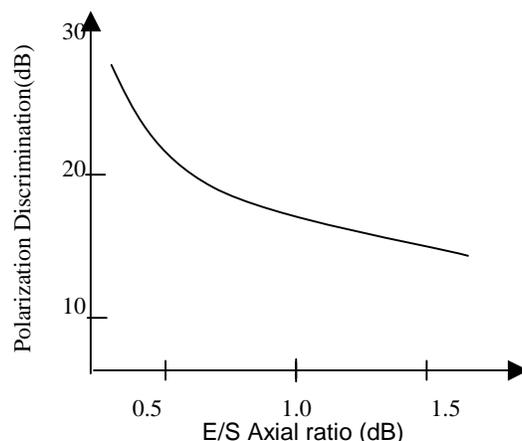
**Figure A.14 Circular Polarization Degradation**
