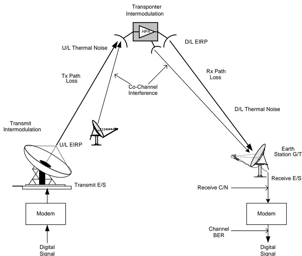
**Figure 9.1 Typical Satellite Link**
