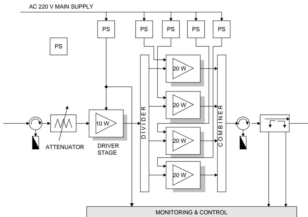
**Figure 5.12 75-Watt SSPA Built from Four 20-Watt SSPA Modules**
