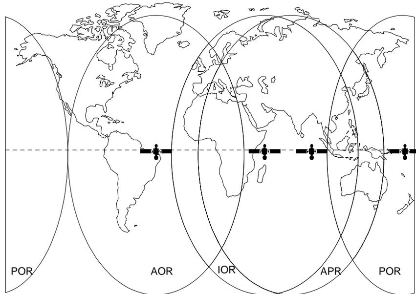
**Figure 1.3 INTELSAT Global Network and Coverage Areas**
