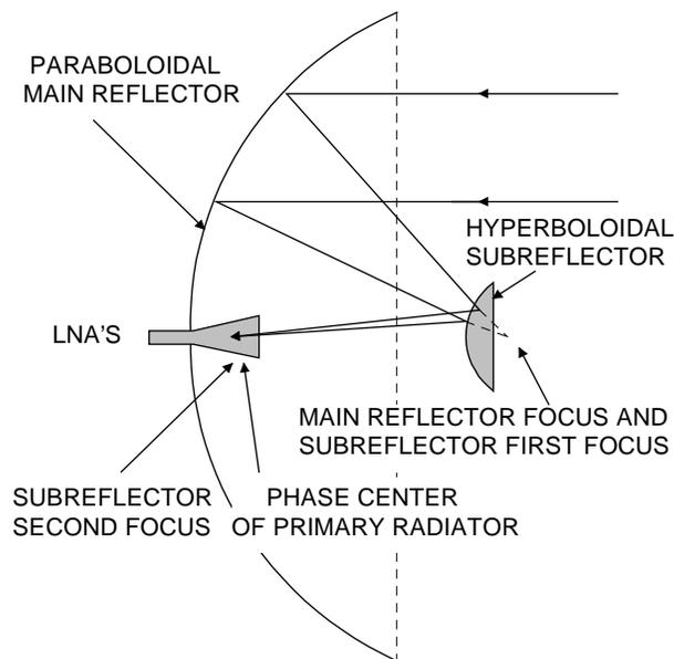
**Figure 3.2 Basic Geometry of a Cassegrain Antenna**
