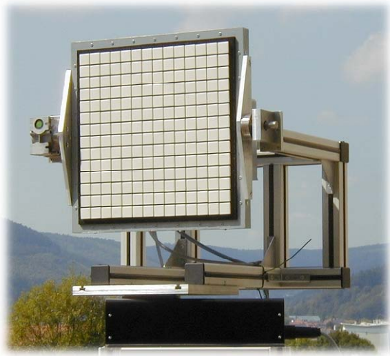
Figure 4: 8x8 URA designed for 5.2 GHz.
