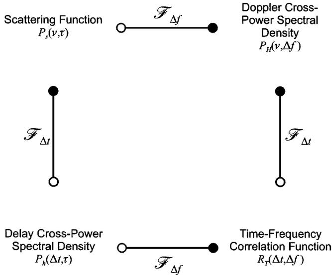
Fig. 2. Correlation functions for time-variant *nondirectional* WSSUS channels and their relations by Fourier transforms.
