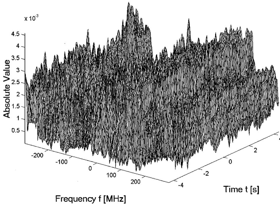
Fig. 6. Time-variant transfer function at a fixed point on the aperture.
