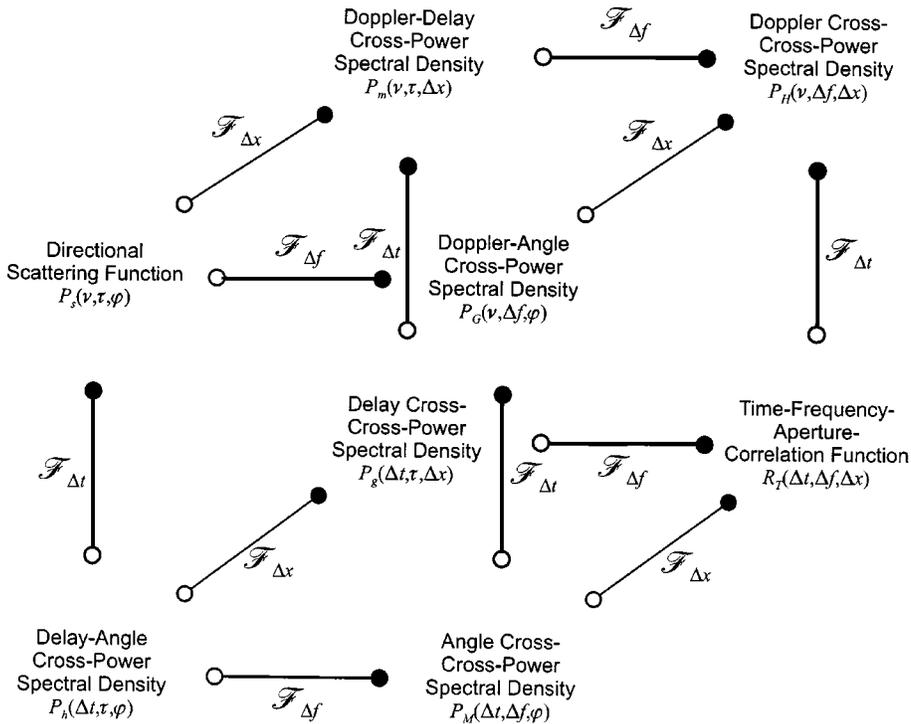
Fig. 5. Correlation functions for time-variant directional WSSUS channels and their relations by Fourier transforms.
