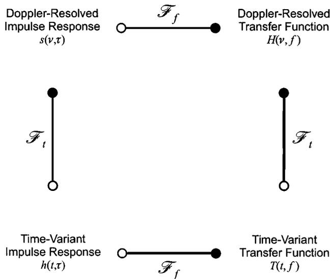
Fig. 1. System functions for time-variant *nondirectional* channels and their relations by Fourier transforms.
