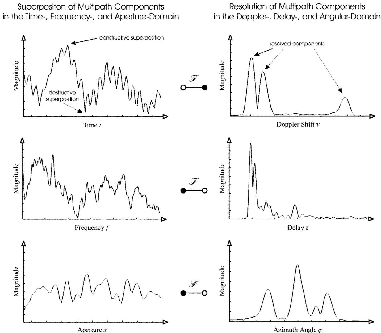
Fig. 3. Superposition and resolution of multipath components in the different domains of directional time-variant channels.
